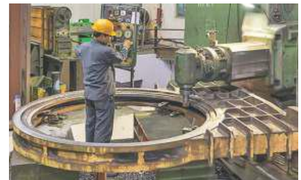
Large floor boring machine for valves up to 3000 mm (120") size.
