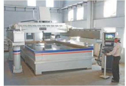
Water jet cutting machine to cut gate up to 100 mm thick.
