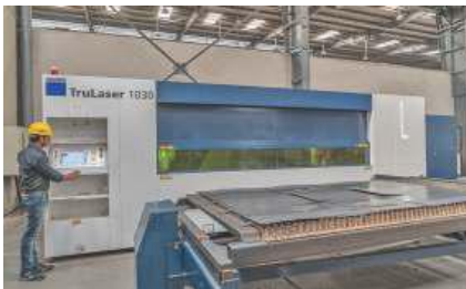
CNC Laser cutting machine to cut gate up to 16 mm thick.
