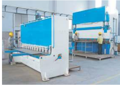
Shearing and bending machine to shear and bend up to 16 mm thick plates.
