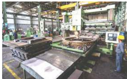
Large CNC milling machine for valves up to 2000 mm (80") size.
