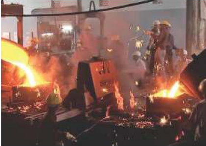
Cast Iron foundry to cast 20 tons castings.
