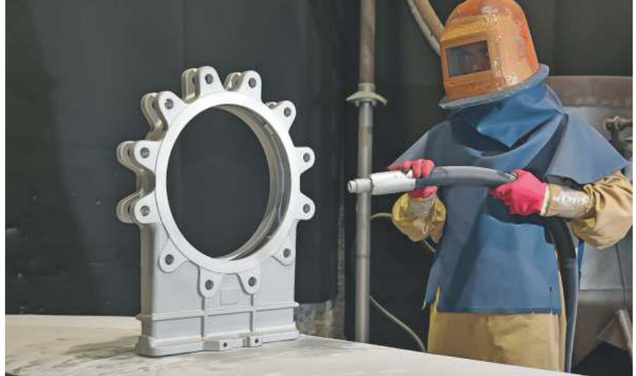
Glass bead / shot blasting for stainless steel valves.
