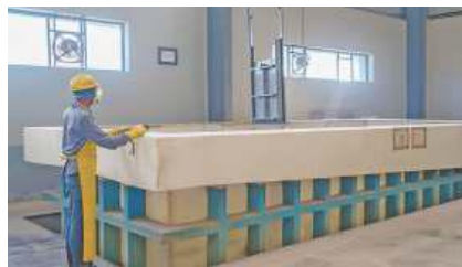
Bath pickling for stainless steel valves.
