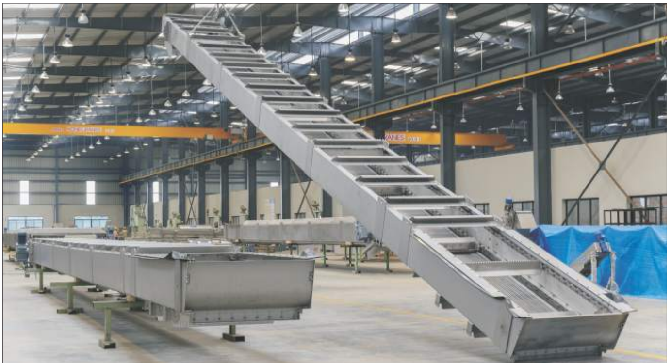
“MM2MM”™ Multirake Screen for DJB Interceptor SPS, Rithala, New Delhi, India
