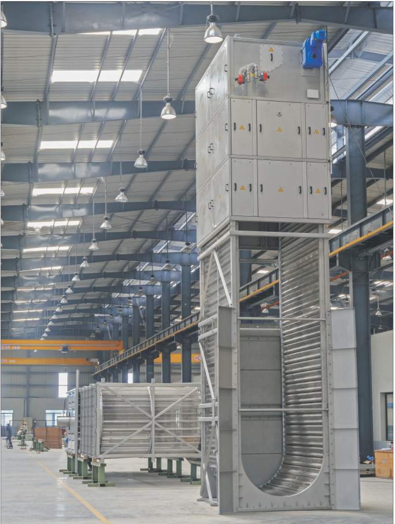
Center flow screen for sea water intake for Tuticorin Power Project, India
