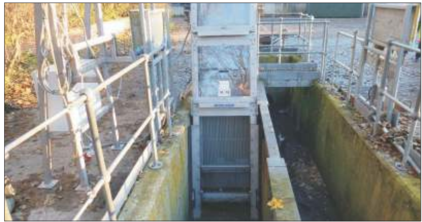
2 mm (0.08”) spacing MM2MM™ screen under testing at National Screen Evaluation Facility, UK
