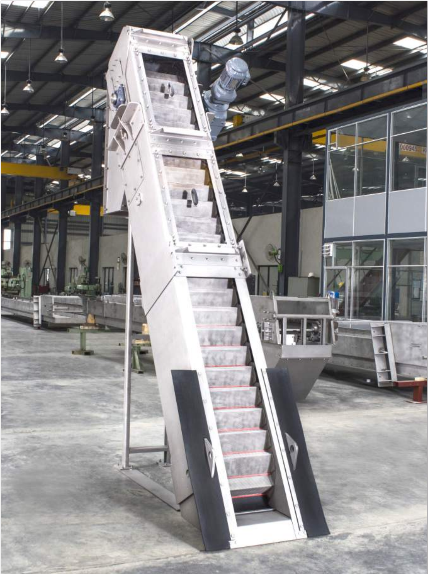
“Per-Scalator” Screen with 4 mm Peforation
