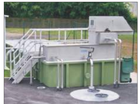
Rotobrush Screen with Grit Removal Mechanism, France
