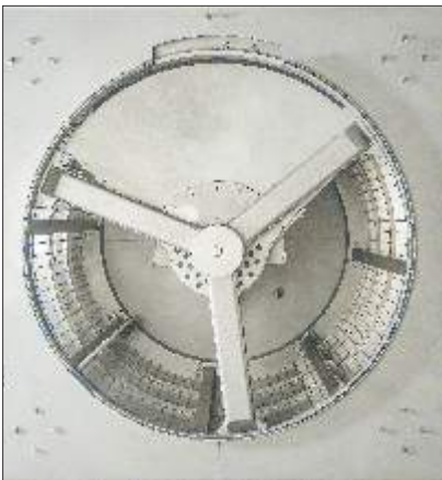
Waste Collection Trough
