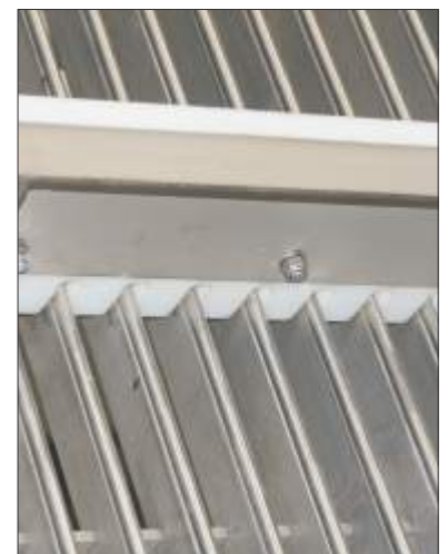
Special Bar Profile with UHMWPE Replaceable Rake
