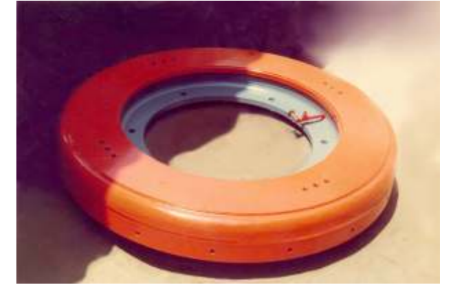
Turn table assembly for SPF-B Clariflocculator
