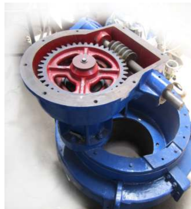
2 stage reduction centre mechanism assembly Type SPT-C Thickener Mechanism
