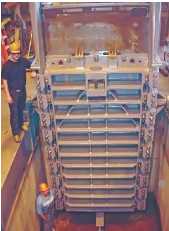
1800 x 3650 mm Cast Iron Slide Gates for Kensico Reservoir, Valhalla, NY, USA
